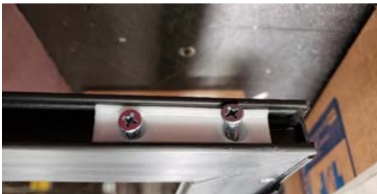
3. Install screws into the bottom door glide
