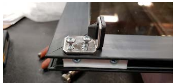
6. Install door stop and screws in reverse order
