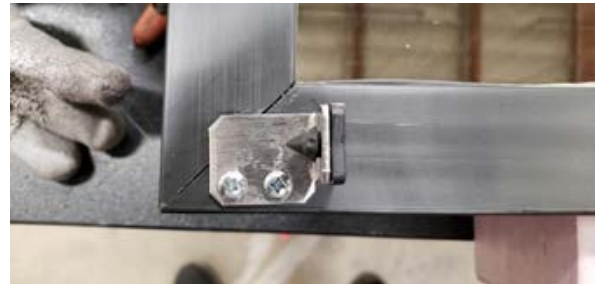
4. To remove door stop, remove both Philips head screws this will also allow you to remove other door glide
